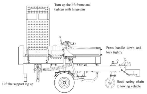
Remember to turn the engine fuel tap off prior to towing to prevent flooding of the engine.
